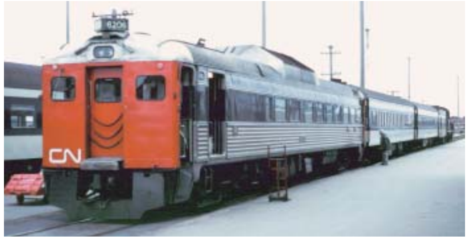
above: RDC-2 No. 6206 is being added to a train of conventional equipment at Moncton. This was the only RDC-2 bought used by CN; it spent most of its service life in the Atlantic Region often coupled back-to-back with No. 6200 (ex-D-200 [ij]). The triangular numberboard on the “B” end was replaced with a combination headlight/numberboard when a diaphragm was installed. Note the Phase Two end windows and pilot.—George Carpenter Collection
