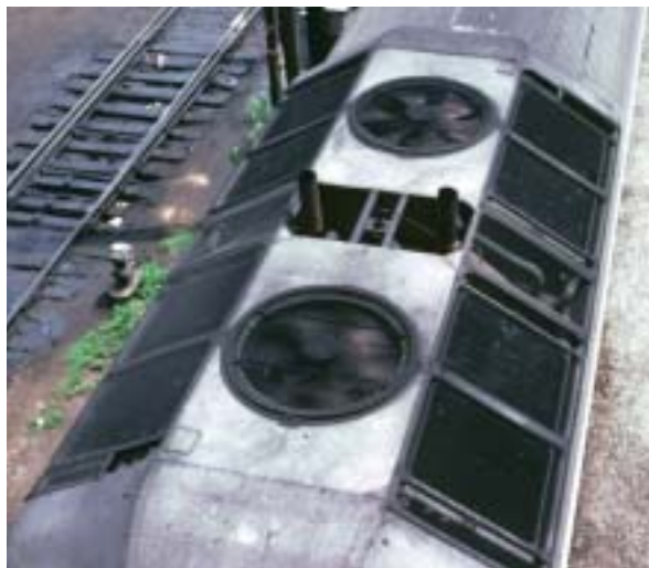
bottom: CNR Railiners had twin exhaust stacks in the roof blister as shown in this 1971 view at Spadina. HO Proto units have a grating here which would have to be removed, and a well and stacks installed. N-scale Kato units have the well and stacks but they are too short and two large in diameter to simulate the CN arrangement. The centre-section grating on the sloping sides has been removed, temporarily, to facilitate radiator maintenance.—Al Lill photo
