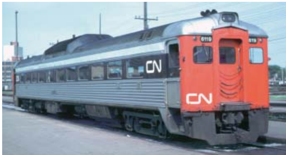
above: Snack-bar equipped RDC-1m No. 6119, shown at Moncton on August 27, 1977, was converted from Phase Two RDC-3 No. 6353 (ex D-353, D-303) when the need for express and mail space diminished.—George Carpenter Collection
