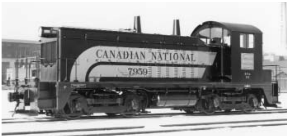
CNR NW2 No. 7959 at EMD in 1947. The CANADIAN NATIONAL RAILWAYS square wafer monograms on the cab sides and Morency Orange hood “flames” accented the black carbody.—EMD photo; Kevin J. Holland Collection
