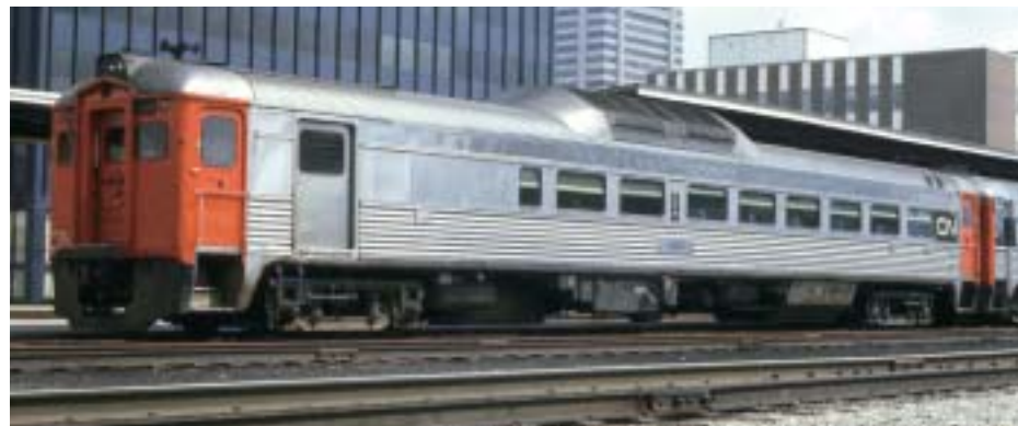
below: CN painted the vestibule doors to cover the CP paint, and retained the bracket for the removable headlight on the end door. CN 6207 at London.—Don McQueen photo
