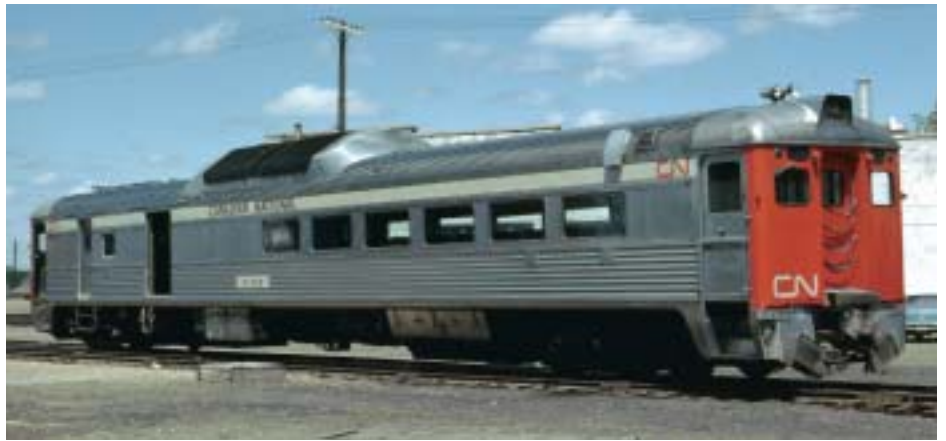
above: The DW&P D-301 with four windows in the passenger compartment was rebuilt as a conventional RDC-3 and renumbered D-355 in 1961. Note the white letter board with the block CANADIAN NATIONAL lettering and orange CN in this June 29, 1964, view at North Regina (after reassignment from Run 78 Prince George–Prince Rupert, B.C.).—Roger Burrows photo
