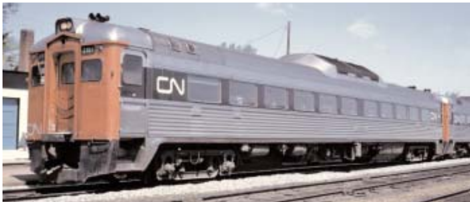
top: Phase Two RDC-1 No. 6105, at Stellarton, N.S., exhibits the full pilot, roof-mounted headlight, smaller end windows and small illuminated numberboards moved to the ends from the car side. A diaphragm retrofitted at this end has been removed. Custom Finishing makes a Phase Two headlight assembly in HO that would help in conversion of a Proto1000 Phase One model. An Athearn shell could be robbed to get the full pilots.—Gary Hatfield photo, courtesy of Matt Kai
