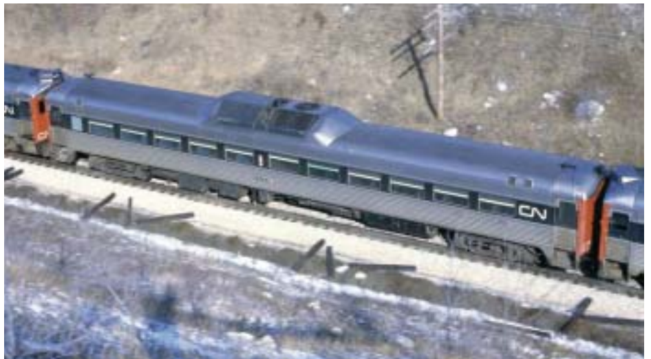
below: Single-engine cabless RDC-9 No. 6006 (ex-B&M) in its usual mid-train position in "Corridor Service" in Southern Ontario.—Don McQueen photo
